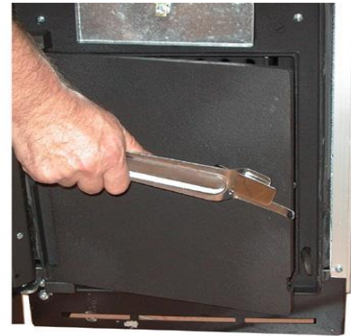
Figure 6 - Opening of the filling door
